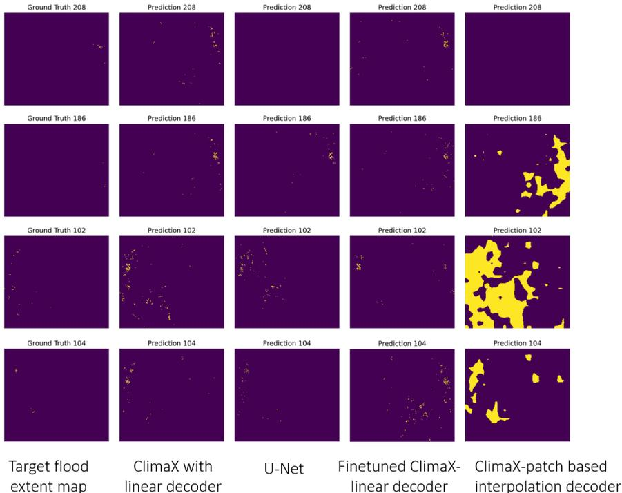
Figure 1: Sample flood extent predictions generated by all evaluated models. The figure qualitatively highlights differences in model performance, particularly in capturing fine-grained flood boundaries and spatial extent.
