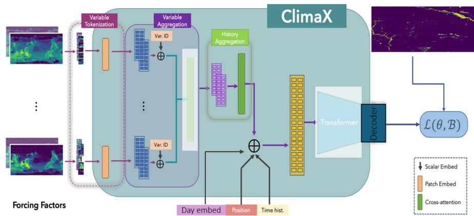
Figure 2: Variant of ClimaX (Nguyen et al., 2023) architecture used in this study for flood extent forecasting.
