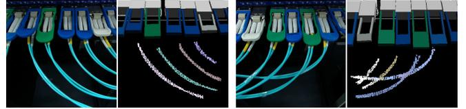
Fig. 7: Local reconstruction results of cables.
