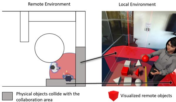
Figure 3: MRTransformer visualizes remote objects as 3D polygons based on overlay computations within collaboration areas, displaying them only when users enter them.
