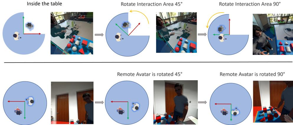
Figure 2: Illustration of rotating a Collaboration Area to move a remote avatar out of occlusion.
