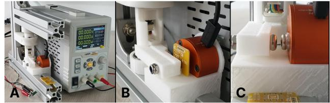
**Figure 18: (A) The ring torque measurement apparatus setup with power supply. (B) Closeup of force measurement unit. The lever arm and force sensor were spaced with two PCB boards. (C) Closeup of torque measurement end effector. Round head Philips screws were fastened to both the lever arm and the force sensor to minimize contact surface area.**
