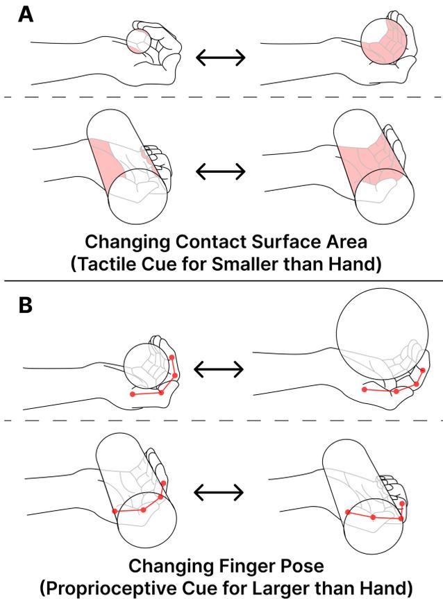
**Figure 1: Analogy of ball of different sizes (top rows of A and B) mapped to proposed finger-repositioning technique (bottom rows of A and B). (A) Illustrates the variation in contact surface area when ball size is fitting or smaller than the hand, with corresponding finger-repositioning around a cylinder that produces similar cues. Likewise, (B) illustrates the variation in proprioceptive cues and corresponding finger-repositioning when the ball size is fitting or larger than the hand.**
