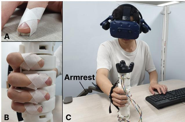
**Figure 7: (A) Closeup of magnet taped to fingertip. (B) Each finger taped and fixated to a ring via magnets. (C) Study setup for Study 1 & Study 2.**
