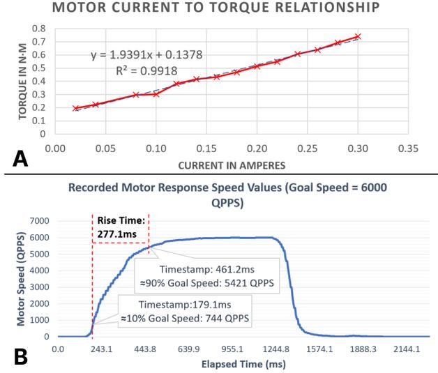
Figure 4: (A) The motor current-torque evaluation plot with dashed trend line. (B) Motor speed evaluation plot with annotated rise time.
