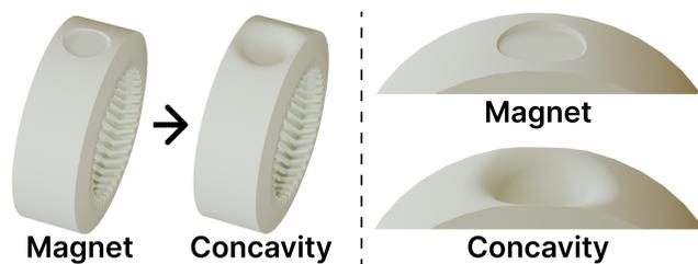
**Figure 17: Alternative approach to fixating fingertips.** By replacing the magnets in the ring with a concavity, the device may be capable of repositioning the fingers without additional fasteners or adhesives.
