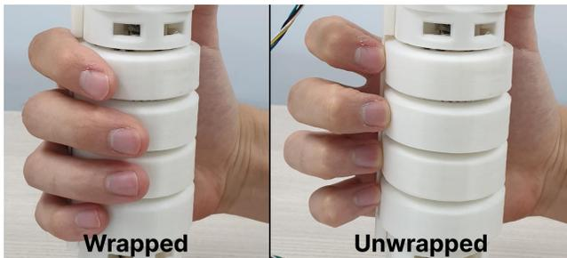
**Figure 3: Example of finger-repositioning via ring mechanism, ranging from wrapped (left) to unwrapped (right) finger pose states.**
