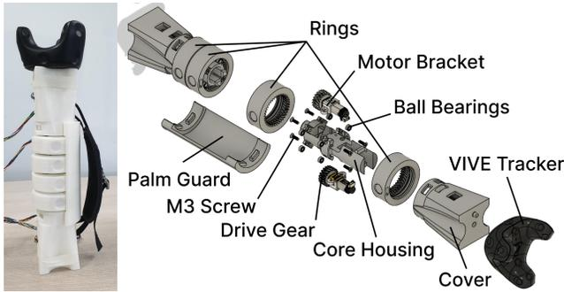
**Figure 2: The finger-repositioning device (left). An exploded view of its assembled components (right).**
