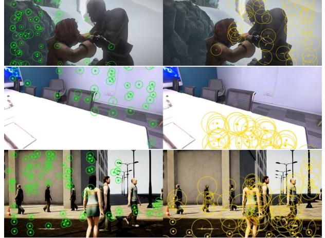
Figure 7. Visualization of point-wise uncertainty measurements. Keypoints with the lowest 20% (left) and highest 20% (right) uncertainty are shown in green and yellow, respectively.
