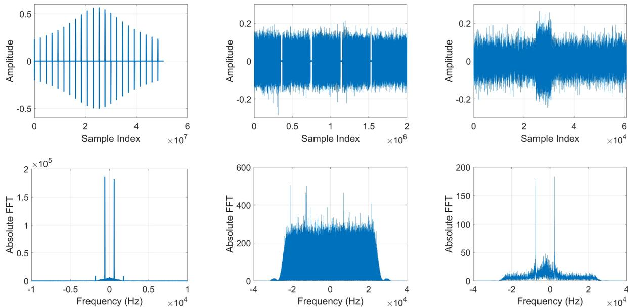
(a) *Emulated signal containing 2-FSK packets transmitted by satellite. Time domain (top) and frequency domain (bottom).* (b) *Signal received at the ground station in real-world. Time domain (top) and frequency domain (bottom).* (c) *Packet found after manual inspection by zooming in the signal. Time domain (top) and frequency domain (bottom).*
