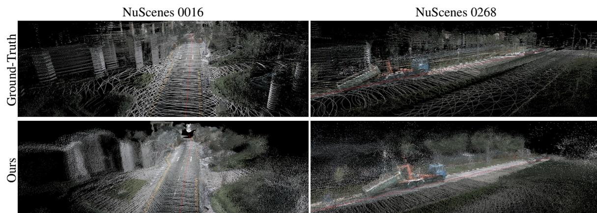
Figure 12. **Qualitative 3D reconstruction results on NuScenes.** We show our 3D reconstruction results alongside the LiDAR ground-truth 3D reconstruction. The ego-vehicle trajectory is marked in red. We observe that our method yields similarly consistent 3D reconstruction results as the LiDAR ground-truth while being denser.
