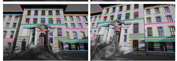
Figure 1: Joint matching of points and lines. Matching feature points often fails in textureless areas (a), while current line matching methods struggle with large view-point changes (c). We propose GlueStick, a network jointly matching points and lines. While none of the methods were trained on the rotations of (a)(b), line matches can guide GlueStick while SuperGlue [50] fails, and vice-versa in (d) where points can complement the line matching. For clarity reasons, we show here only the correct matches.
