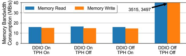
**Fig. 5:** Memory bandwidth consumption by PCIe-bench’s DMA write with different DDIO/TPH settings.
