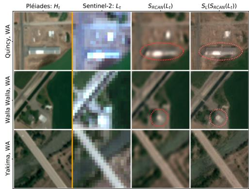
**Fig. 1:** RCAN with and without matrix completion sharpening: The dotted lines highlights features that are significantly sharper and less blurry after matrix completion sharpening.
