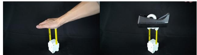
Figure 6: The actuator maximum holding load is 1379 g at the extended state (25 cm height)
