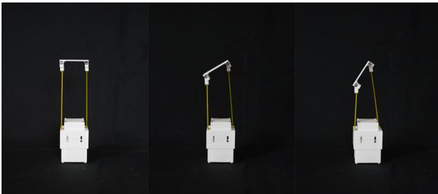
**Figure 8: The cap can tilt up to 60 degrees.**
