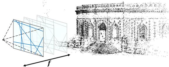
**Figure 1:** Our method jointly estimates absolute pose and focal length of uncalibrated cameras from privacy preserving line features. We also present a solution for bootstrapping maps from scratch using four views.
