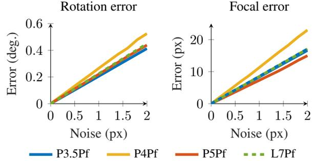
**Figure 4: Noise Sensitivity.** The graphs show the median errors in the rotation (*Left*) and the focal length (*Right*) for varying noise levels. The errors in the translation are qualitatively similar and can be found in the supplementary material.
