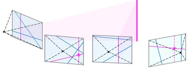
**Figure 2: Initialization.** We solve a projective 2D-SfM problem with consistently aligned lines. Points in the projective reconstruction project onto aligned lines in the images. Intersecting random lines with the aligned projections allow us to recover the 2D key points for a subset of the original line correspondences.
