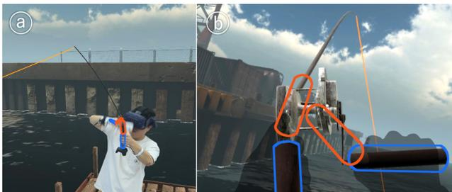
**Figure 12: In the *fishing rod* application, each controller expresses different features of the rod. The left controller renders bending of the rod, while the right simulates the motion of a winch.**
