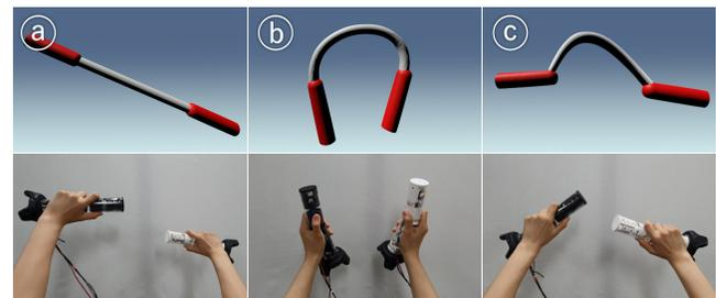
**Figure 5: Visual and haptic renderings of three example bonds: (a) Rigid, (b) Soft, and (c) Dynamic.**
