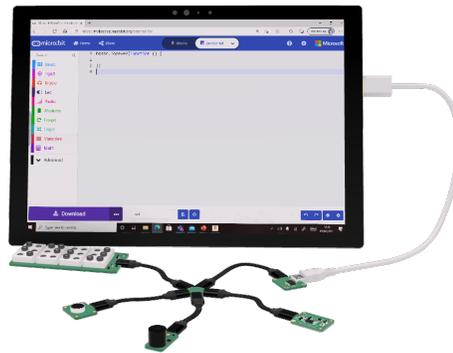
Fig. 1. A conceptual vision of a BVI accessible physical computing environment, showing a web-based accessible programming editor and hardware modules connected together by a reversible, low-cost multi-wire cable. Modules include: a braille display module, a sounder module for audio output, a haptic module for vibrational feedback, an accelerometer for orientation detection, and a re-programmable microcontroller module that controls operation of all other modules.
