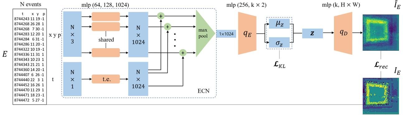
**Figure 2:** Architecture of the event variational autoencoder (eVAE). Events from the bytestream are directly processed by a PointNet-styled network to compute individual features. Temporal embeddings are added to these features and the *max* operation results in a global context vector. This is then projected into a latent space, and subsequently decoded into an ‘event image’.
