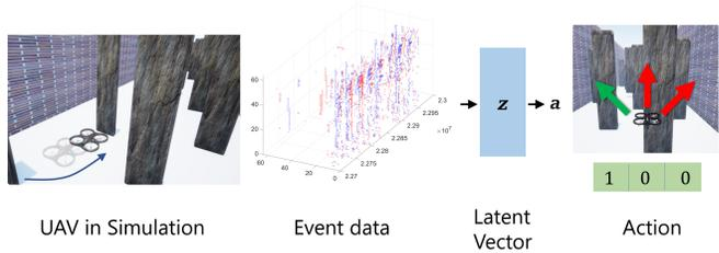
**Figure 1:** Event cameras provide fast, asynchronous measurements of per-pixel log luminance changes. We present a representation learning technique that can encode context from such spatiotemporal event bytestreams. Subsequently, we show these low-dimensional representations are beneficial for learning visuomotor policies through a simulated UAV obstacle avoidance task.
