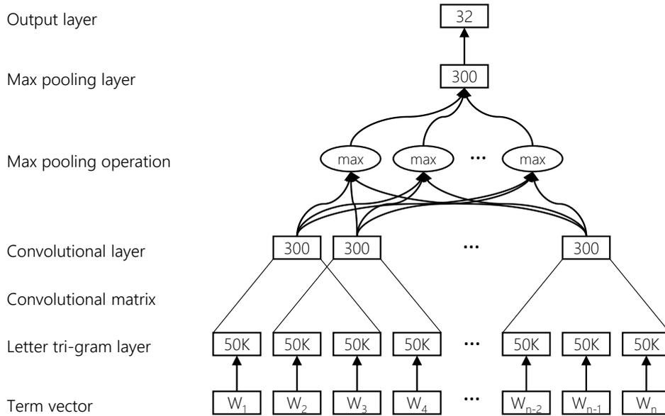
**Figure 7.1:** Architecture of the CDSSM. The model has an input layer that performs the *word hashing*, a convolutional layer, a max pooling layer, and an output layer that produces the final semantic vector representation of the query.
