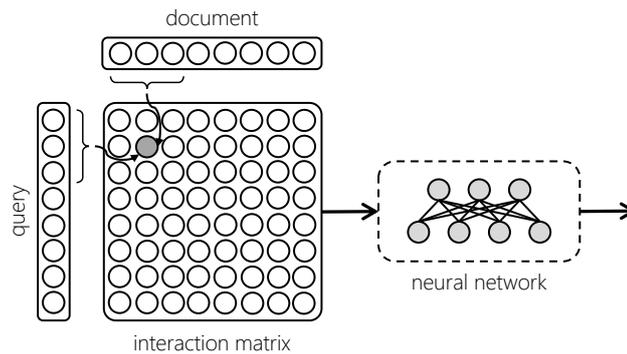
**Figure 3.19:** Schematic view of an interaction matrix generated by comparing windows of text from the query and the document. A deep neural network—such as a CNN—operates over the interaction matrix to find patterns of matches that suggest relevance of the document to the query.
