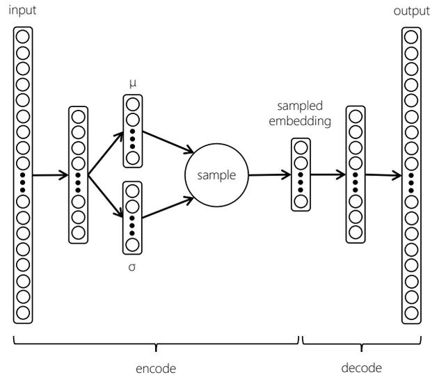
**Figure 3.18:** Instead of directly generating an encoded representation, variational autoencoders sample the latent vector from the generated vector of means  $\mu$  and standard deviations  $\sigma$ . This local variation forces the model to learn a smoother and more continuous latent space.
