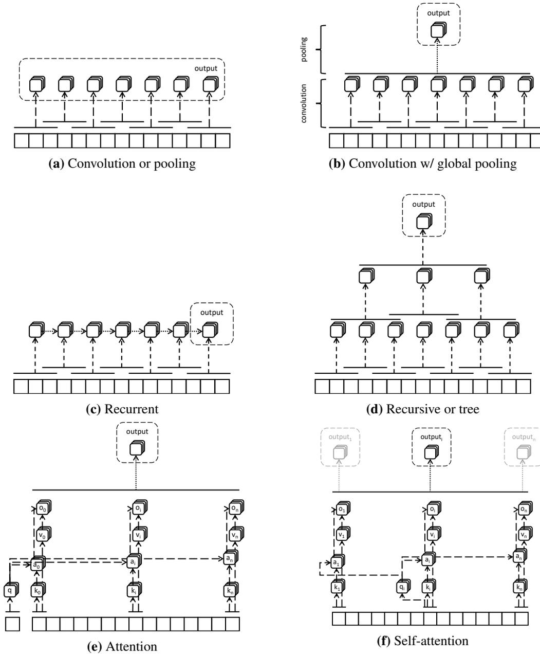
**Figure 3.16:** Standard shift-invariant neural architectures including convolutional neural networks (CNN), recurrent neural networks (RNN), pooling layers, tree-structured neural networks, attention layer, and self-attention layer.
