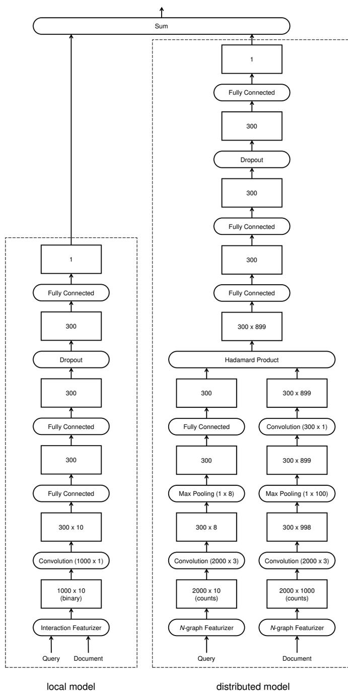
**Figure 4.2:** The Duet network is composed of the local subnetwork (left) and the distributed subnetwork (right). The local subnetwork takes an interaction matrix of query and document terms as input, whereas the distributed subnetwork learns embeddings of the query and the document text before matching. The parameters of both subnetworks are optimized jointly during training. Hyperparameters such as  $n_{hidden}$  and  $n_{pool}$  shown as in the document ranking task.
