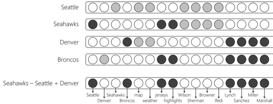
**Figure 3.7:** A visual demonstration of term analogies via simple vector algebra. The shaded circles denote non-zero values. Darker shade is used to highlight the non-zero values along the vector dimensions for which the output of  $\vec{v}_{Seahawks} - \vec{v}_{Seattle} + \vec{v}_{Denver}$  is positive. The output vector is closest to  $\vec{v}_{Broncos}$  as shown in this toy example.
