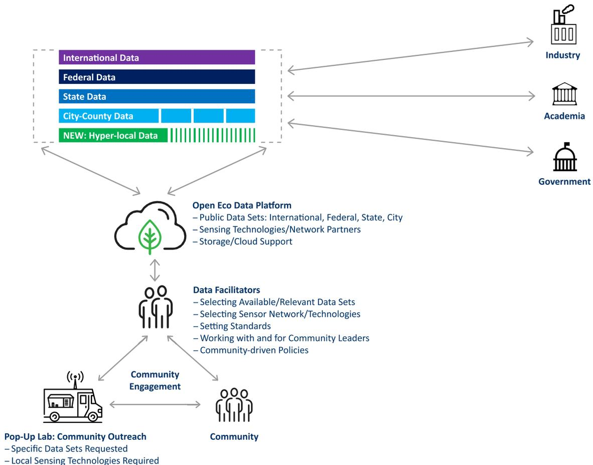
Figure 4: Open eco data platform design
