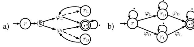
Fig. 5.  $SBFA(r)$ ;  $r = r_L \& r_D$ ;  $r_L = .*[a-z].*$ ;  $r_D = .* \backslash d.*$ .
