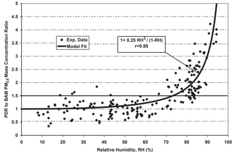
Two-hour averaged pDR to BAM  $\text{PM}_{2.5}$  concentration ratio as a function of relative humidity.
