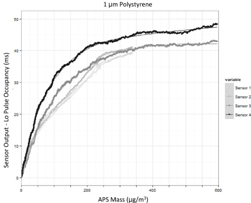
Lab chamber study with consistent synthetic particles
