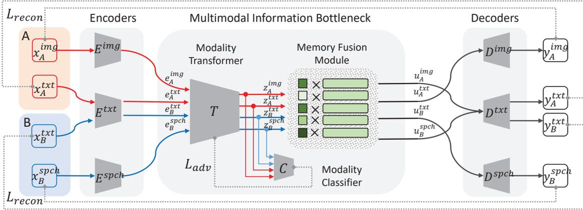
Figure 2. Our model consists of modality-specific encoders  $E^{(\cdot)}$  and decoders  $D^{(\cdot)}$ , and a multimodal information bottleneck that learns to represent different modalities in a shared embedding space. We train the model end-to-end using two disjoint datasets involving image, text, and speech (A and B) by solving cross-modal reconstruction tasks. The modality classifier  $C$  is used only during training.
