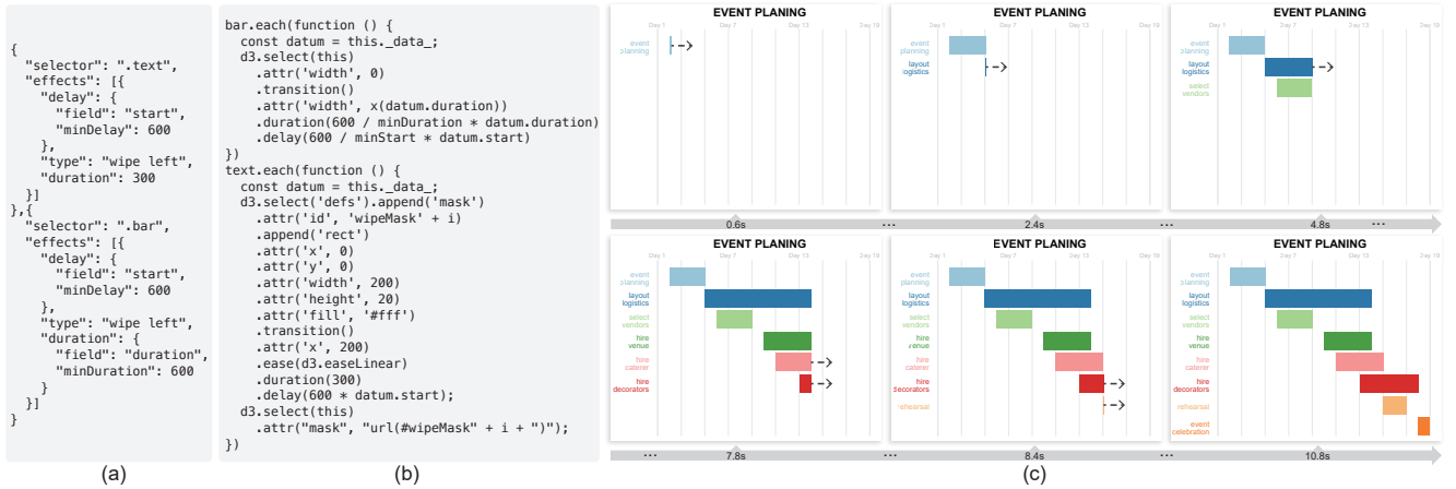
Figure 5: The animation of creating a Gantt chart designed by using Canis and D3. (a) The partial specification of Canis where two marks “text” and “bar” are selected and specified with same effect but different timing parameters; (b) the partial specification of D3, where two functions are provided for animating each type of marks; and (c) six snapshots of the animation, where the arrow indicates the text and bar movement direction. Some chart titles and legends are partially occluded because of the overlap between snapshots.
