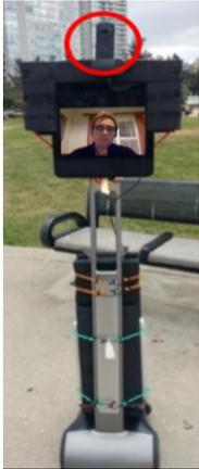
**Figure 1:** Beam telepresence robot with 360° camera (circled) attached. This camera streams to a remote user who can view the robot's surroundings in VR.
