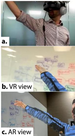
**Figure 4:** VROOM: the remote user gesturing at a white board. **a.** Remote (VR) user's action. **b.** Remote (VR) user's view. **c.** Local (AR) user's view.
