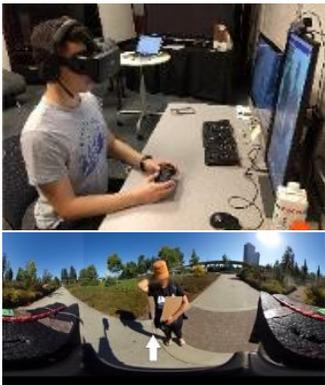
**Figure 2:** The remote user operating the telepresence robot using a VR interface (top), immersing themselves in the faraway location (bottom).
