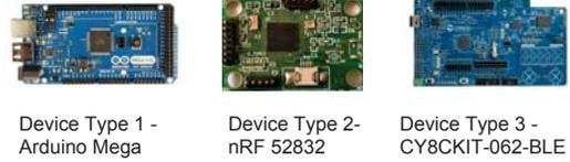
Fig. 8: Different device types used for evaluation.
