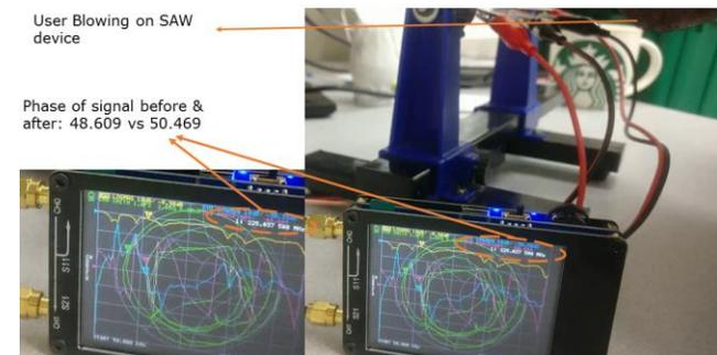
**Figure 3:** When a user blows on the SAW device our vector network analyser shows a distinct phase change of  $\sim 2^\circ$ .
