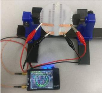
**Figure 4:** SAW IDTs are connected to input and output channels of a low cost vector network analyzer.
