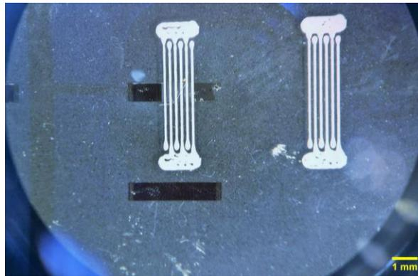
**Figure 6:** A Voltera DIW printed SAW device. The traces that make up the IDTs are  $100\mu\text{m}$  wide.
