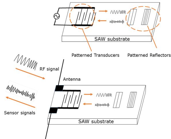
**Figure 1:** (a, top) The typical structure of a SAW device, based on an interdigitated transducer (IDT) and similarly structured reflectors patterned on top of the SAW crystal substrate. (b, bottom) A SAW device connected to an antenna: an RF signal is transmitted to SAW device wirelessly and ultimately the return signal is reflected back.
