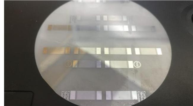
**Figure 2:** Our custom-made SAW devices on a lithium niobate wafer. We patterned 8 devices on a single wafer using traditional photolithography.
