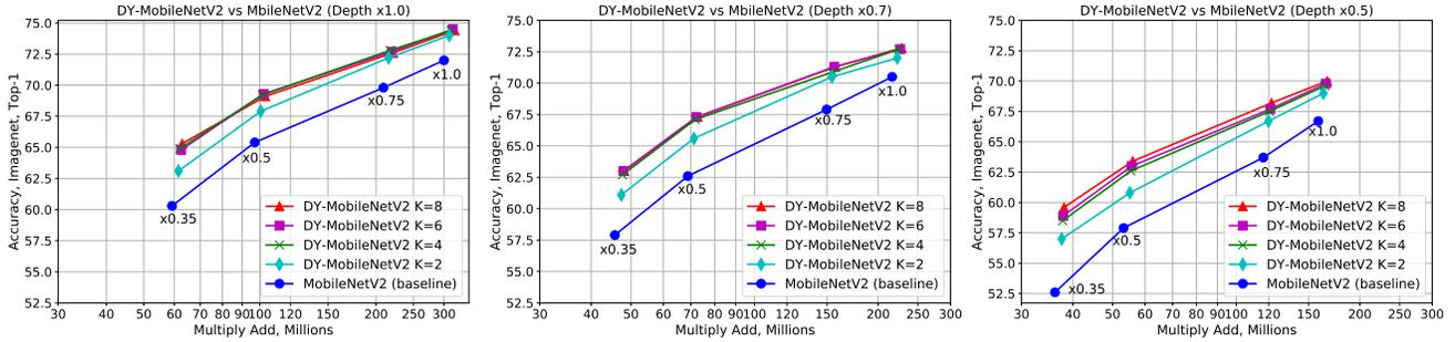
Figure 6. **The number of convolution kernels ( $K$ )** in DY-MobileNetV2 with different depth and width multipliers. **Left**: depth multiplier is 1.0, **Middle**: depth multiplier is 0.7, **Right**: depth multiplier is 0.5. Each curve has four width multipliers  $\times 1.0$ ,  $\times 0.75$ ,  $\times 0.5$ , and  $\times 0.35$ . Dynamic convolution outperforms its static counterpart by a clear margin for all width/depth multipliers. Best viewed in color.
