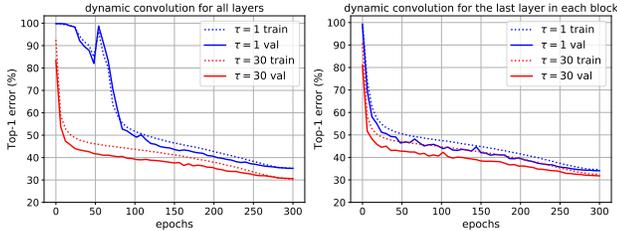
Figure 5. Training and validation errors for using different soft-max temperatures. **Left:** using dynamic convolution for all layers. **Right:** using dynamic convolution for the last layer in each bottleneck residual block. We use DY-MobileNetV2 with width multiplier  $\times 0.5$ , and each dynamic convolution layer has  $K = 4$  convolution kernels. Best viewed in color.
