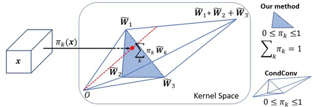
Figure 4. Illustration of constraint  $\sum_k \pi_k(\mathbf{x}) = 1$ . It compresses the space of aggregated kernel  $\sum_k \pi_k \tilde{W}_k$  from two pyramids (used in CondConv [37]) to a triangle. A red line is compressed into a dot by normalizing attention sum. Best viewed in color.
