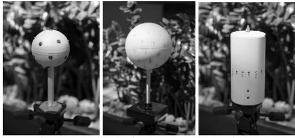
(a) 16 channels 115 mm spherical (b) 64 channels 200 mm spherical (c) 16 channels 115 mm cylindrical
