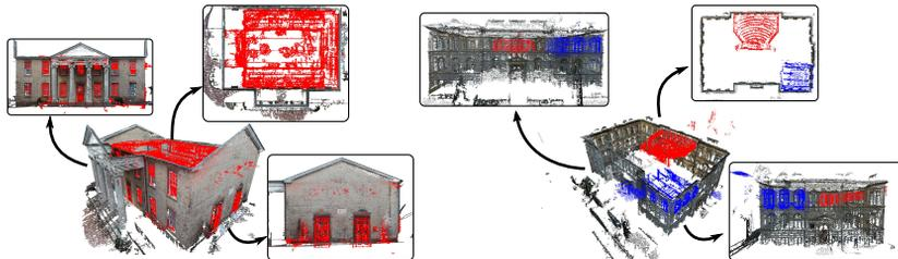
**Fig. 1.** The proposed method aligns disconnected Structure-from-Motion reconstructions of the inside and outside to produce a single 3D model of a building. Our approach also handles incomplete reconstructions and multiple indoor models (*c.f.* right model)
