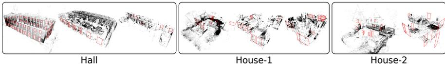
Fig. 6. Window detections obtained as described in Sec. 4
