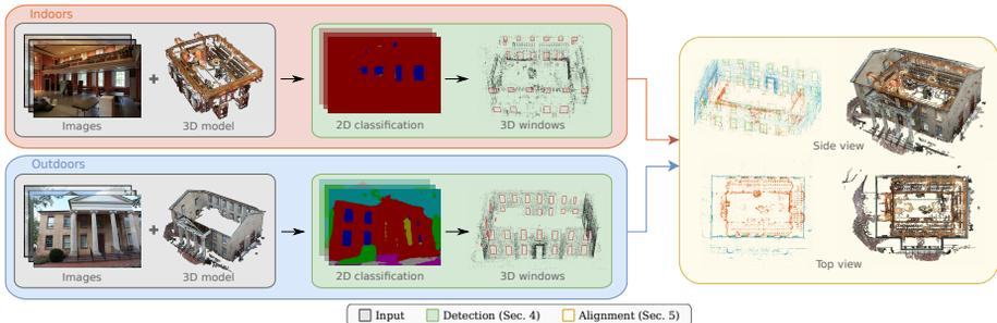
**Fig. 2.** Given SfM reconstructions of indoors and outdoors together with their input images, we leverage per-pixel semantic classification to detect windows in 3D. These windows are then used to compute a registration between both scenes that maximizes the number of aligned windows while avoiding that the models intersect each other
