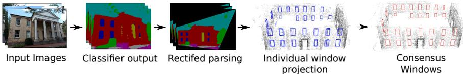
**Fig. 3.** The proposed 3D window detection pipeline
