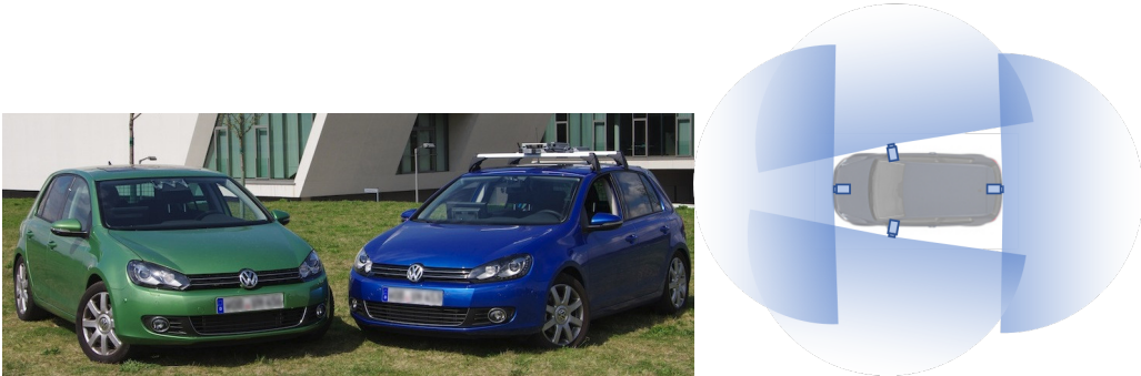
Figure 2: (left) The two cars from the V-Charge project. (right) The cameras are mounted in the front and back and in the side view mirrors.
