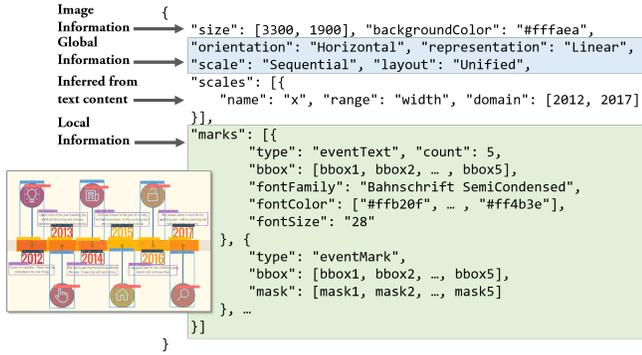
Fig. 11: The extensible template can be organized in a reusable document. The **bbox** is a tuple of  $(top, left, width, height)$ . The **mask** is a byte array with shape  $width \times height$ .
