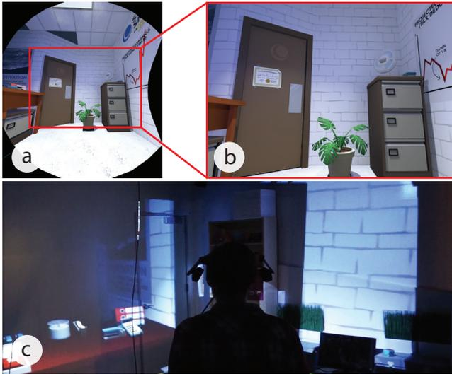
**Figure 11: The HMD user's in-game view projection mapped onto physical surfaces from a co-located spectators point of view. a) the left eye view, b) the companion window view, and c) the projection mapped content.**
