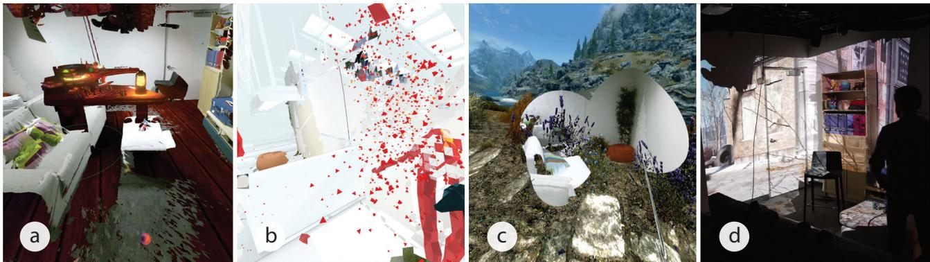
**Figure 1: RealityCheck blends the VR player's real world with the virtual world. A real time 3D reconstruction of the player's room is integrated into the VR title's rendering pipeline to allow: a) proper 3D hidden surface removal (*Waltz of the Wizard*), b) collision estimation (*SUPERHOT VR*), c) a flashlight into reality using controllers (*Skyrim VR*), and d) co-located spectatorship through projection mapping (*Fallout 4 VR*).**
