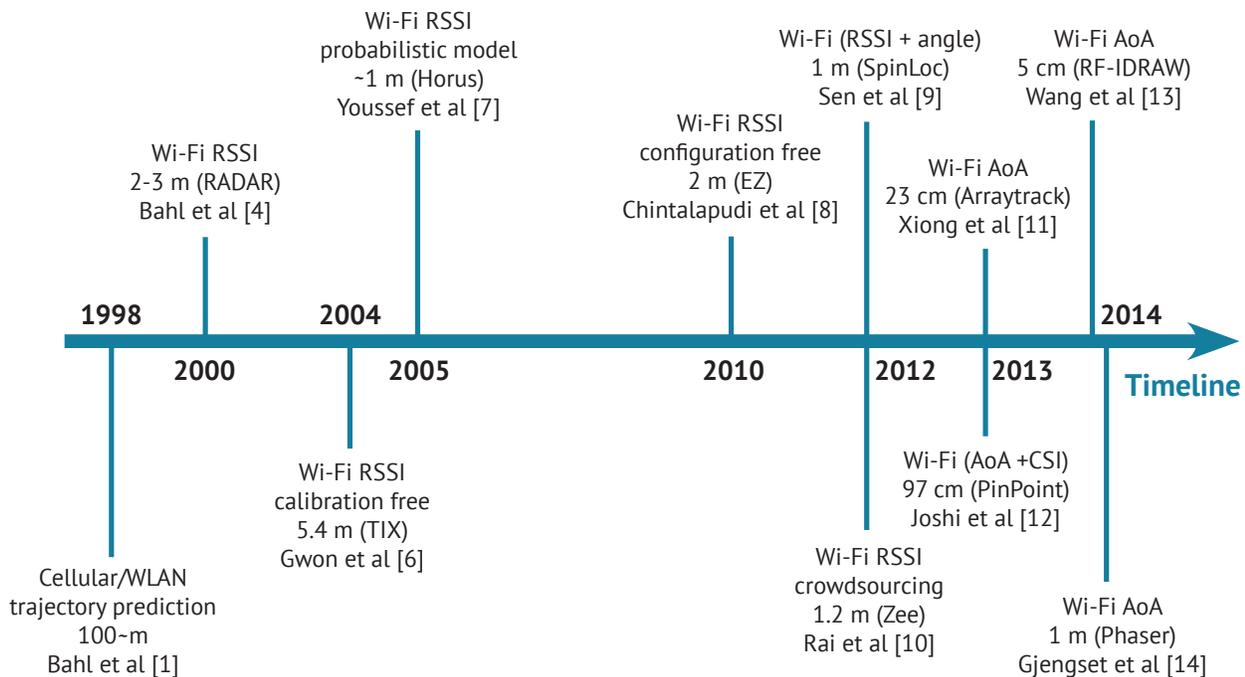
**FIGURE 2.** A sample of the indoor localization techniques and their target accuracy as claimed by the inventors (RSSI: Received Signal Strength Information; AoA: Angle of Arrival; CSI: Channel State Information).
