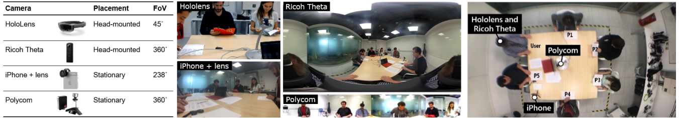
Figure 1. Left: Camera placement and field-of-view (FoV); Center: Sample images from each camera; Right: Test scenario set-up.
