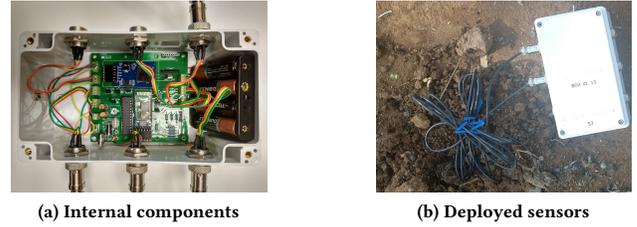
Figure 12: IoT sensor node deployed in agricultural farms.
