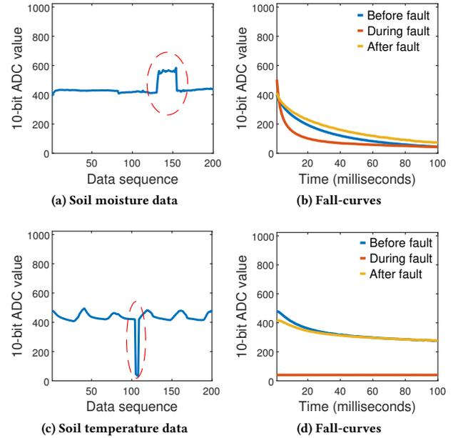
**Figure 14: Spike fault and its corresponding Fall-curves.**
