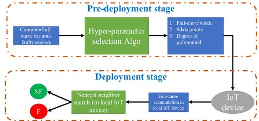
Figure 10: Block diagram of Fall-curve processing pipeline.
