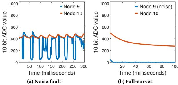
Figure 16: Noise fault and its corresponding Fall-curves.
