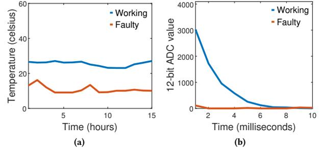
Figure 9: Non-faulty vs faulty digital DHT sensor.
