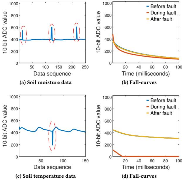
**Figure 13: Short fault and its corresponding Fall-curves.**
