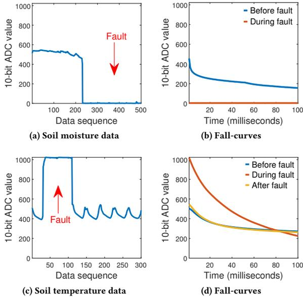
Figure 15: Stuck-at fault and its corresponding Fall-curves.
