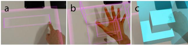
Fig. 7. Blueprint extrusion app. (a) The user draws a blueprint with their finger. (b) They use an in-air open-hand gesture to extrude it, using hand height to set the extrusion distance. (c) The user closes their hand to lock-in the extrusion.
