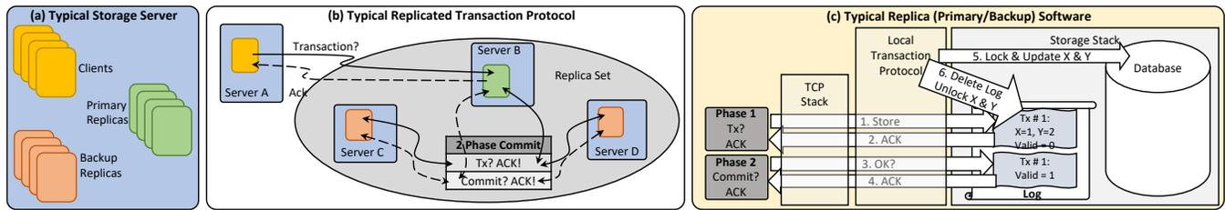
**Figure 1: Servers in data center storage systems typically co-locate 100s of replicas of many tenants to improve utilization. This increases latency due to frequent context switches when replica processes, network and storage stacks continually vie for the CPU. Unfortunately, it is not economically viable for 100s of replica processes to be pinned on dedicated cores and poll.**
