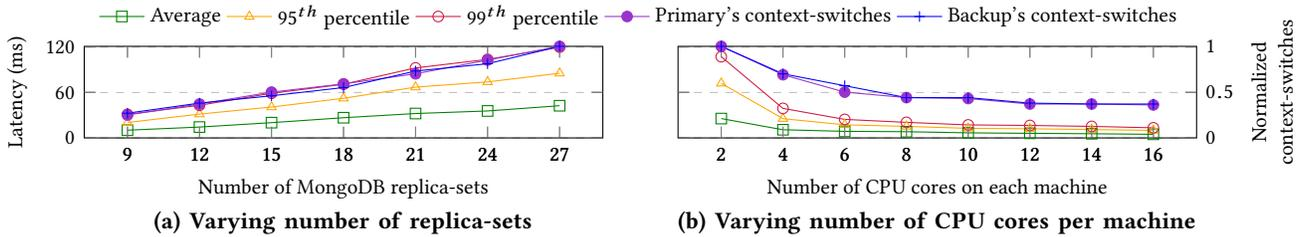
**Figure 2: Analyzing the impact of CPU on MongoDB’s latency distribution using YCSB. Normalized context-switches is the number of context-switches for each configuration divided by the maximum for all configurations in each chart.**
