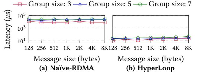
Figure 10: 99<sup>th</sup> percentile latency of gWRITE with different group sizes compared to Naïve-RDMA.
