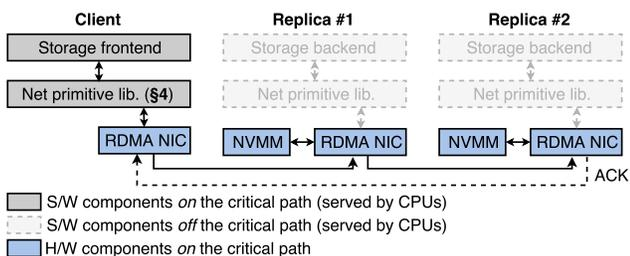
**Figure 3: Storage system architecture with HyperLoop.**
