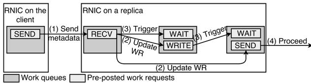
**Figure 7: Datapath of gMEMPCPY primitive.**
