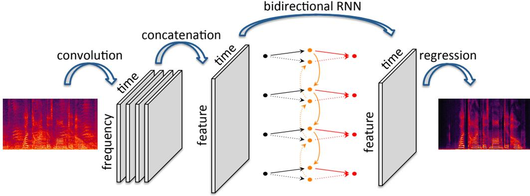
**Fig. 1:** Model architecture. EHNNet consists of three components: noisy spectrogram is first convolved with kernels to form feature maps, which are then concatenated to form a 2D feature map. The 2D feature map is further transformed by a bidirectional RNN along the time dimension. The last component is a fully-connected network to predict the spectrogram frame-by-frame. EHNNet can be trained end-to-end by defining a loss function between the predicted spectrogram and the clean spectrogram.
