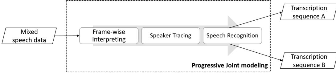
Fig. 1. *The Proposed System Framework. The single monolithic structure (the dashed line box) that predicts independent targets for each speaker, proposed in [14], is improved through modularization (three solid line boxes) and pretraining. Self-transfer learning and multi-output sequence discriminative training are conducted on modularly initialized layers.*
