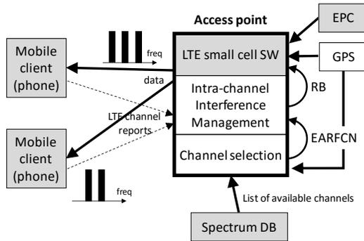
**Figure 3: CellFi architecture overview.** The shaded blocks denote unmodified existing components (parts of LTE network stack and TVWS database) and the white blocks are new components introduced by CellFi.
