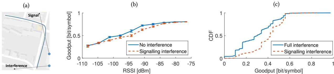
**Figure 7: Outdoor LTE interference experiment setup (a), the difference between no interference and signalling-only interference (b) and the difference between signalling-only interference and data interference (c).**
