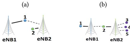
**Figure 5:** Lines reflect associated clients to access points while dashed lines reflect interference. (a) Information asymmetry with two total channels. eNodeB 1 overestimates his share because it cannot sense UE 2. (b) Information asymmetry with 4 total channels. eNodeB 2 has a share of 1, and while eNodeB 1 can increase his share to 3, it only reserves his fair-share, i.e., 2 channels because it does not know how many subchannels 2 is using (1 due to UEs 3-5)
