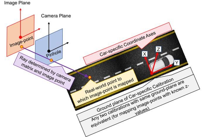
Figure 3: Using geometries extracted from a vehicle, AutoCalib calibrates the camera w.r.t the car specific GCS.
