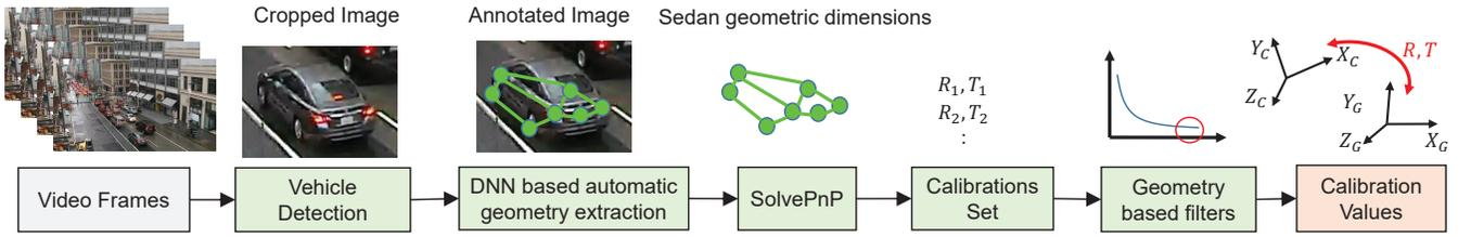
Figure 1: AutoCalib pipeline for automatic calibration of traffic cameras.
