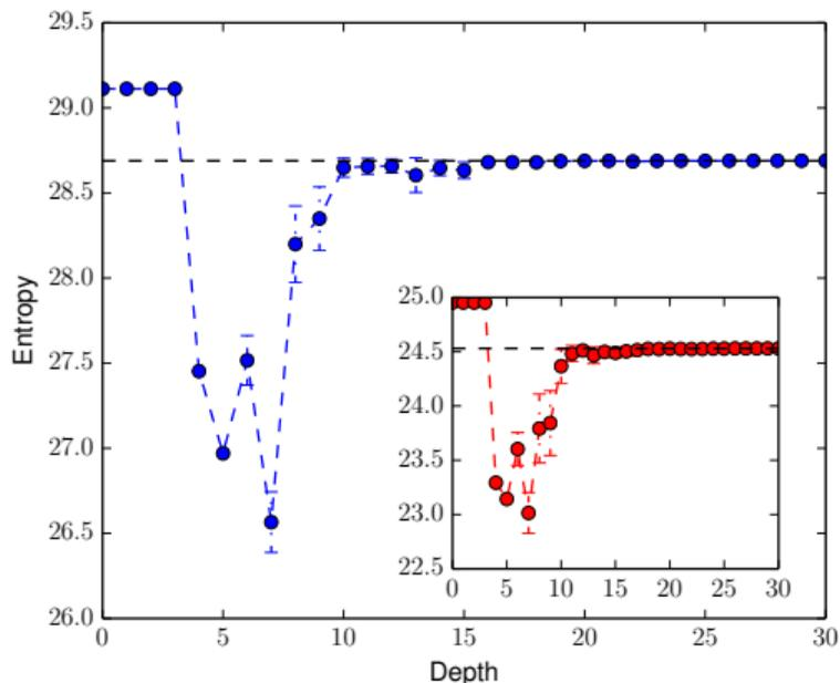
Figure: Depth required for PT distribution. Dashed line is known entropy for PT. 2D circuit  $7 \times 6$  qubits. Inset  $6 \times 6$  qubits.
