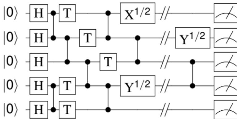
Figure: Vertical lines correspond to controlled-phase gates .
