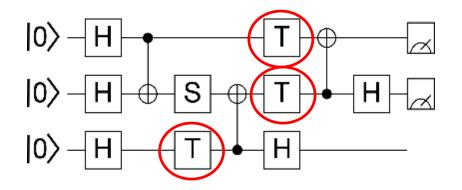
$$T=\left[egin{array}{cccc} 1 & 0 \ 0 & e^{i\pi/4} \end{array}
