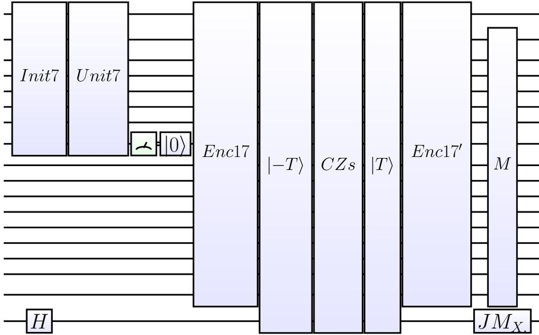
FIG. B.2. Pipelined circuit using  $[[17, 1, 5]]$  code described in section IA 2.
