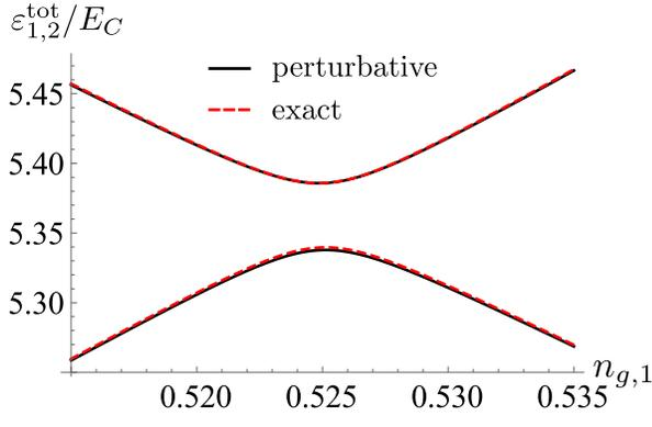
FIG. 16. Agreement between perturbative (solid black) and exact (dashed red) parity-dependent energies  $\varepsilon_1^{\text{tot}}$  and  $\varepsilon_2^{\text{tot}}$  in units of  $E_C$ . We use the parameter values  $N_{g,a} = 0$ ,  $n_{g,2} = n_g^*$ ,  $p = p_{12}p_{34} = 1$ ,  $\varepsilon_{C,a} = 10E_C$ ,  $h = E_C/2$ ,  $\varepsilon_M = E_C/2$ ,  $t_1 = 0.1E_C$ , and  $t_{j \neq 1} = 0.2E_C$ .
