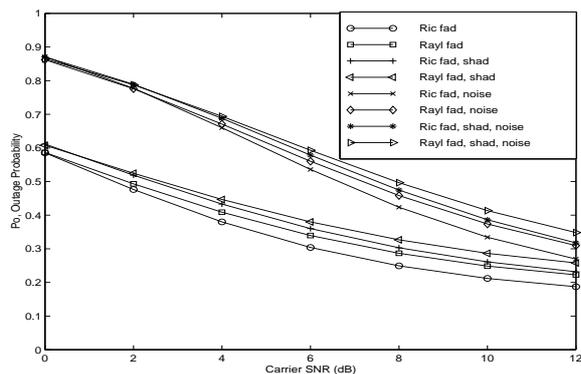
Figure 3:  $P_o$  vs. carrier SNR for Rayleigh and Ricean fading channels with and without lognormal shadowing,  $L=3$  interference sources.
