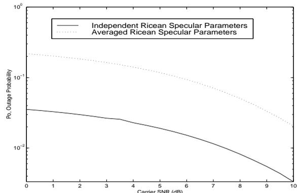
Figure 1:  $P_o$  vs. carrier SNR for Ricean fading channels with independent and dependent specular parameters.
