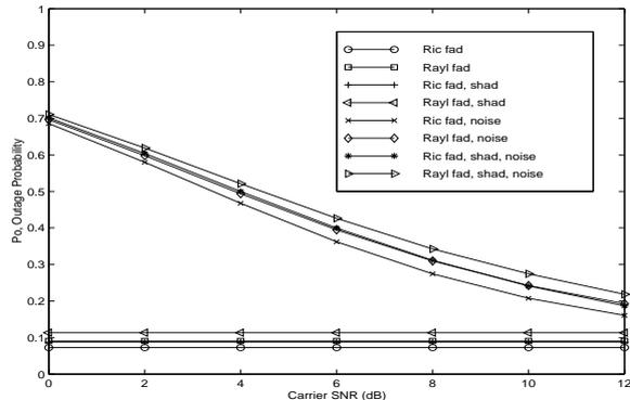
Figure 2:  $P_o$  vs. carrier SNR for Rayleigh and Ricean fading channels with and without lognormal shadowing,  $L=1$  interference source.
