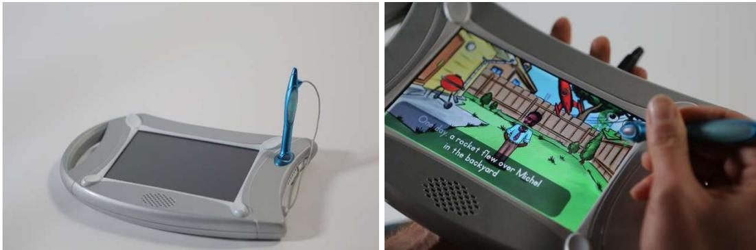
**Figure 17. The prototype hardware (2007). a) The prototype device; b) Story Baker running on the device.**
