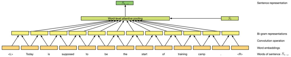
Our model **CRSum+SF** is shown in Figure 2, where we combine  $v(S_t)$ ,  $f_{pc}(v(S_t), v_{pc}(S_t))$  and  $f_{fc}(v(S_t), v_{fc}(S_t))$  with four basic Surface Features (**SF**) listed in Table 2. Then we apply a MultiLayer Perceptron (MLP) [12, 41] as the decoder to transform the features into a single value as the final salience score to  $S_t$ , as shown in Eq. 5:
