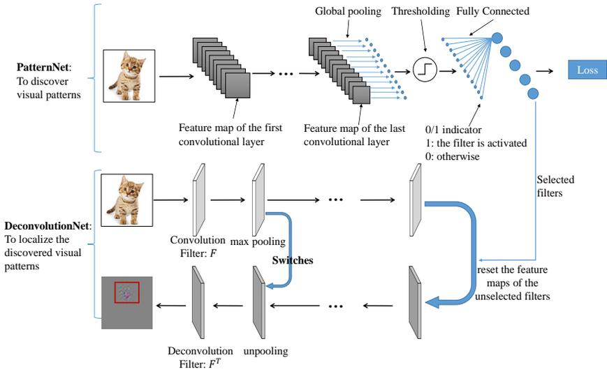
**Fig. 2.** PatternNet Architecture. The proposed system use PatternNet to discover visual patterns. The visual patterns are represented by a set of filters. Once the visual patterns are discovered, a deconvolutional neural network is used to localize the location of the visual pattern in the input image.
