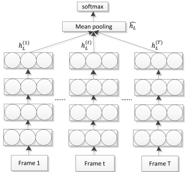
Figure 1. Overall diagram of the proposed utterance-level DNN.
