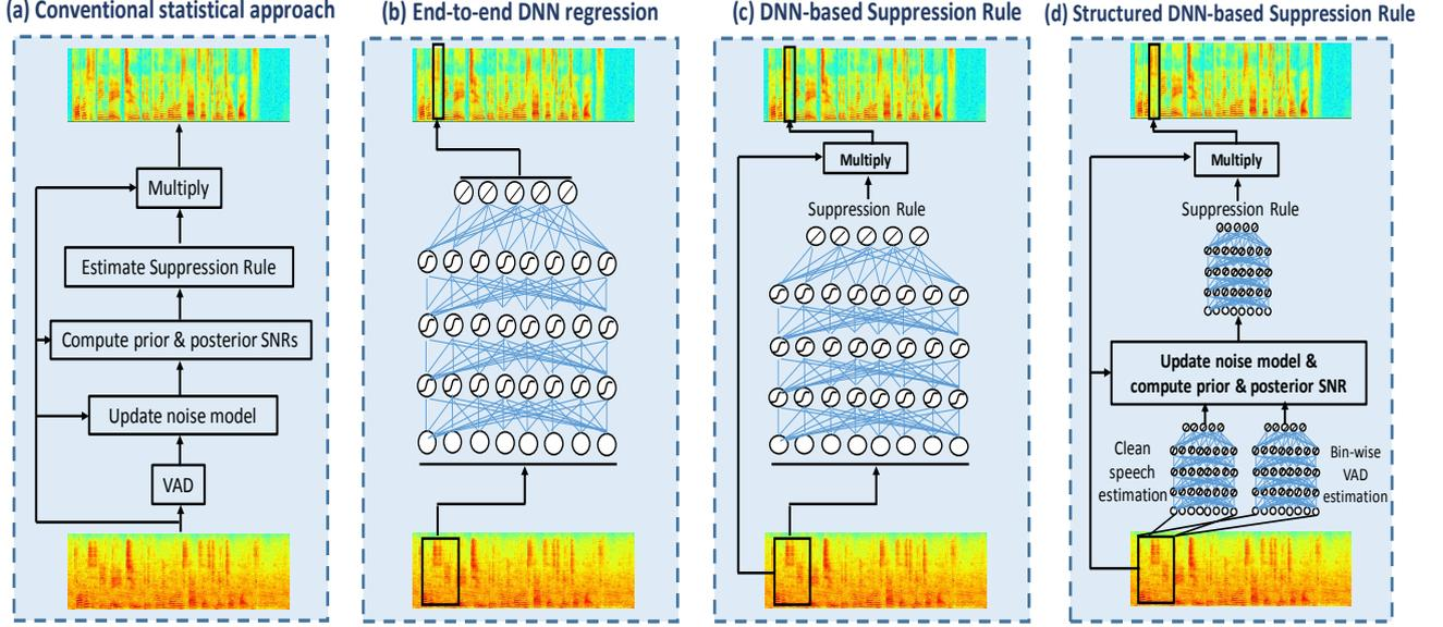
Figure 1: Different architectures for DNN-based speech enhancement: (a) Statistical noise suppression. (b) Enhancement by end-to-end DNN regression from noisy spectral features to clean features. (c) Estimating bin-wise suppression gain directly by a DNN. (d) Employing separate DNNs replacing the different components of conventional suppression gain estimation.
