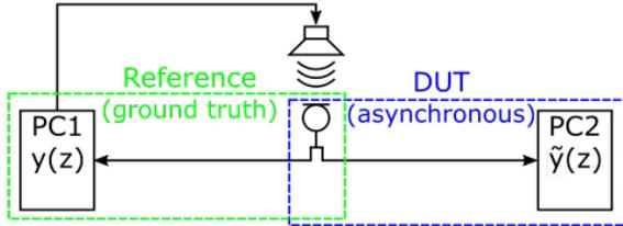
**Fig. 2.** Experimental setup consisting of clock-synchronous reference system (PC1) and asynchronous DUT (PC2).
