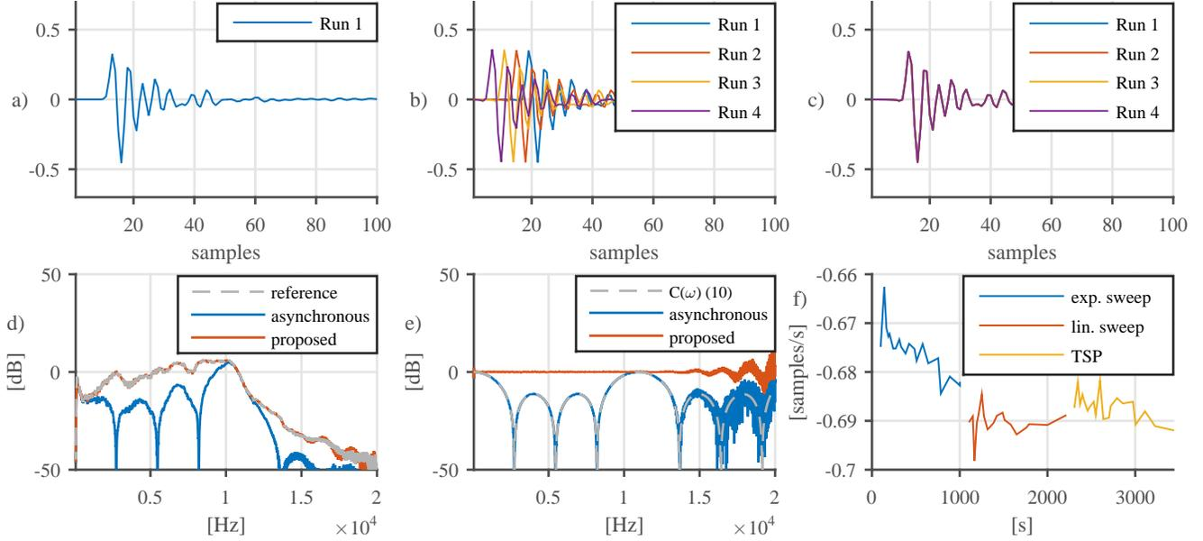
**Fig. 1.** Temporal and magnitude response of ground-truth reference IR (a, d) and asynchronous IR measurement with four repetitions without clock drift compensation (b, d) and with proposed drift compensation (c, d); e) shows the magnitude response error of the asynchronous IR measurement; f) shows estimated drift rates using various test signals over time.
