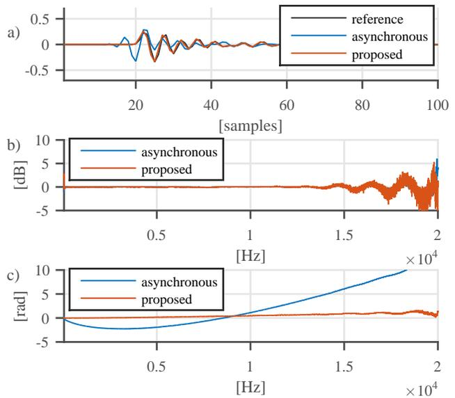
**Fig. 3.** a) Asynchronous IR estimated with a single, long exponential sweep, and with four repetitions of a short sweep after the proposed clock drift compensation; b) magnitude and c) phase response of the equivalent drift filters, given in (11).
